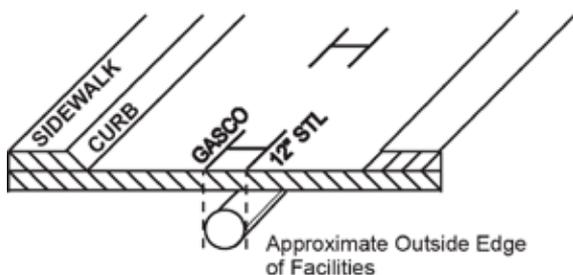
These examples indicate an operator's 12 in. facility. When a facility can be located or toned separately from other subsurface installations of the same type, it is marked as a single facility.
