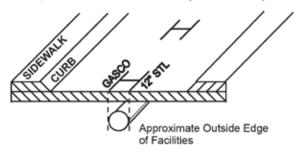
These examples indicate an operator's 12 in. facility. When a facility can be located or toned separately from other subsurface installations of the same type, it is marked as a single facility.
